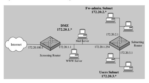
Fig. 3. The network topology of the example
