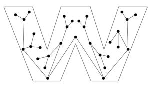
Fig. 11. Drawing of a 31-node complete binary tree by our algorithm inside a W-shaped polygon
