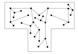
Fig. 9. Drawing of a 31-node complete binary tree by our algorithm inside a T-shaped rectilinear polygon
