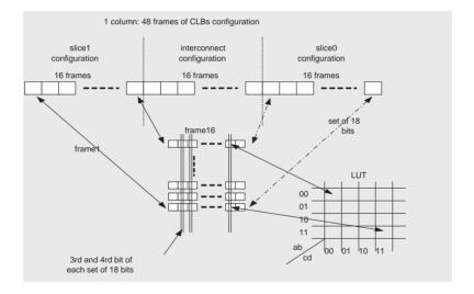
Fig. 1. Positions in the frames of the LUT configuration bits
