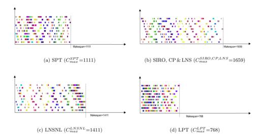
Fig. 6. Problem (3): Gantt charts of dispatching rules applications for the instance  $G_1 = 15 \& G_2 = 12$
