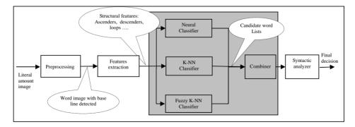
Fig. 1. Global system architecture
