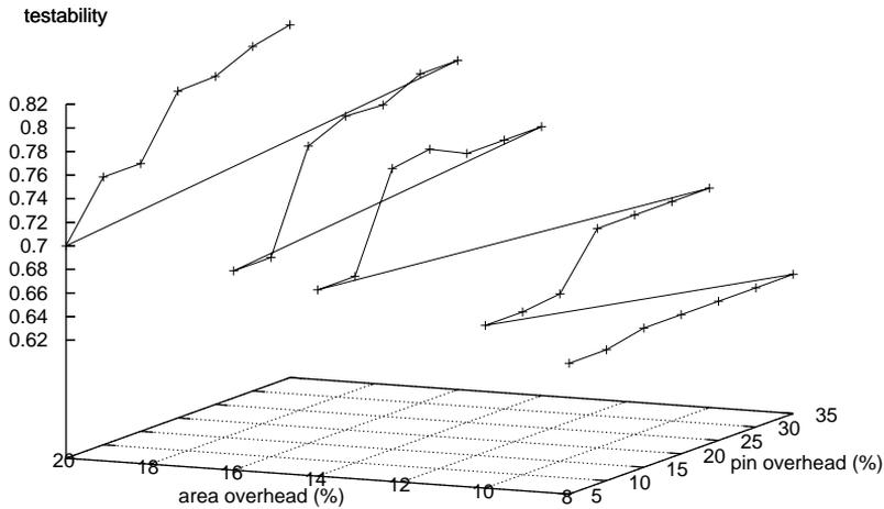
Fig. 9. Visualisation of testability distribution in *Diffeq* scan layout state-space
