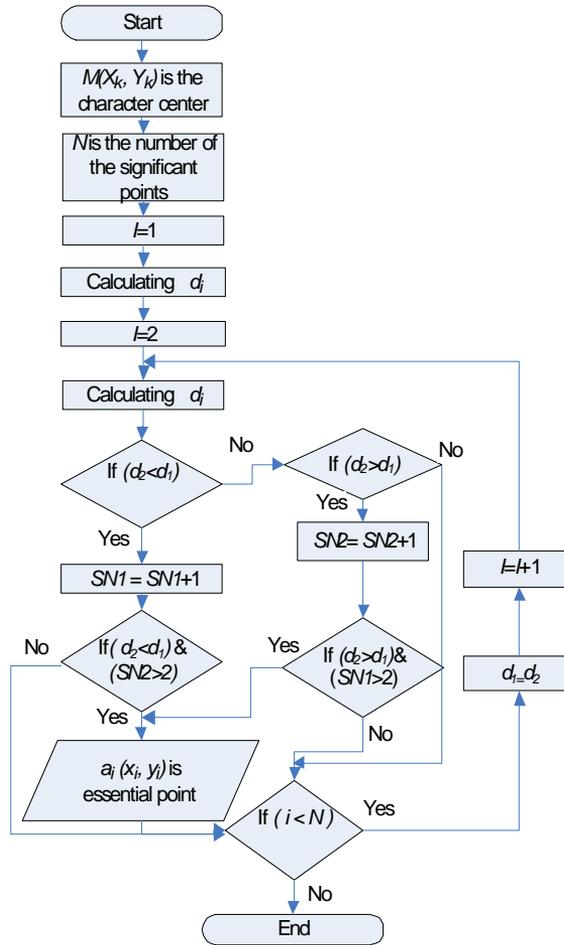
Fig. 5. The flow chart of the essential points verification
