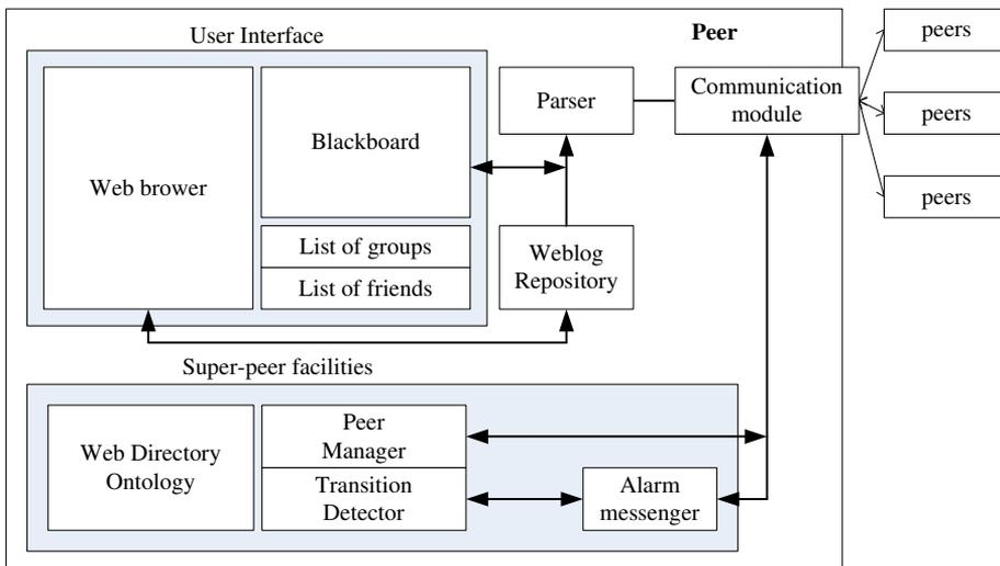
Fig. 5. System architecture based on blackboard module
