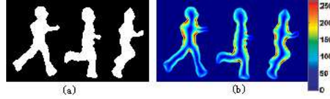
Fig. 1. The \|\nabla U(x, y)\| image for the silhouette images of example postures. a) The example postures; b) The \|\nabla U(x, y)\| image for the postures. The level set (from dark blue to red) is used to indicate the intensity of pixels in the images.
