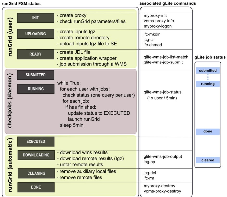
Fig. 4. States of the runGrid command and checkJobs daemon as described in the text. We also indicate the gLite commands associated to each state.
