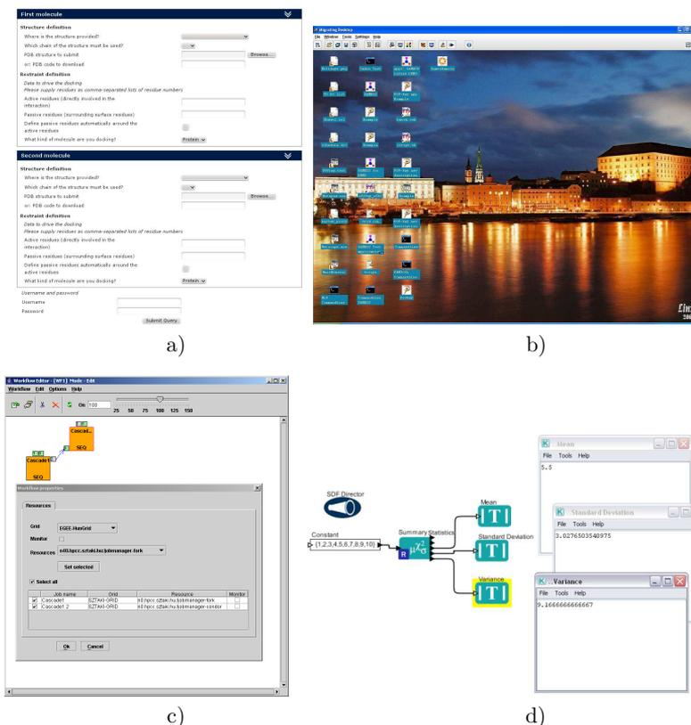
Fig. 2. a) Easy interface to the HADDOCK docking program. b) Default main Migrating Desktop window. c) P-GRADE job editor. d) Kepler simple workflow definition.
