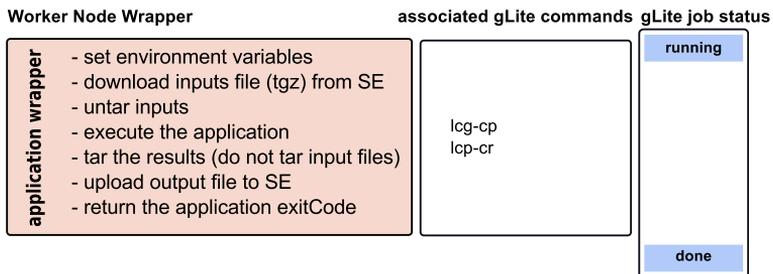
Fig. 5. In the Worker Node the user application is replaced by the application wrapper that downloads the inputs from the Storage Element, executes the user application, compresses the outputs and uploads the file to the Storage Element. Finally, the exit code returned to the WMS is the same the user application returned.
