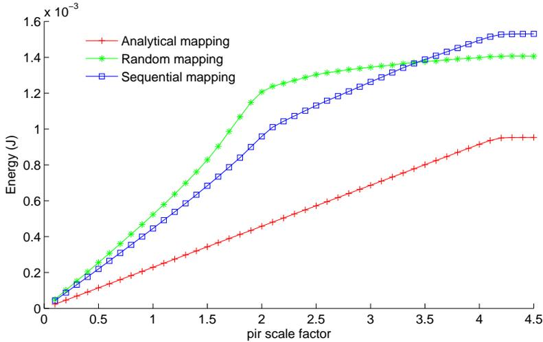
Fig. 22. Energy consumption required by different mappings for the shuffle traffic distribution
