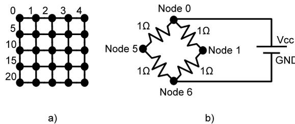
Fig. 2. a) A 2-D network topology b) Equivalent circuit for going from Node 0 to Node 6
