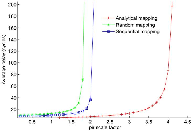
Fig. 19. Latencies provided by different mappings for the bit-reversal traffic distribution
