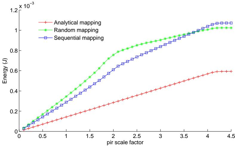
Fig. 20. Energy consumption required by different mappings for the bit-reversal traffic distribution
