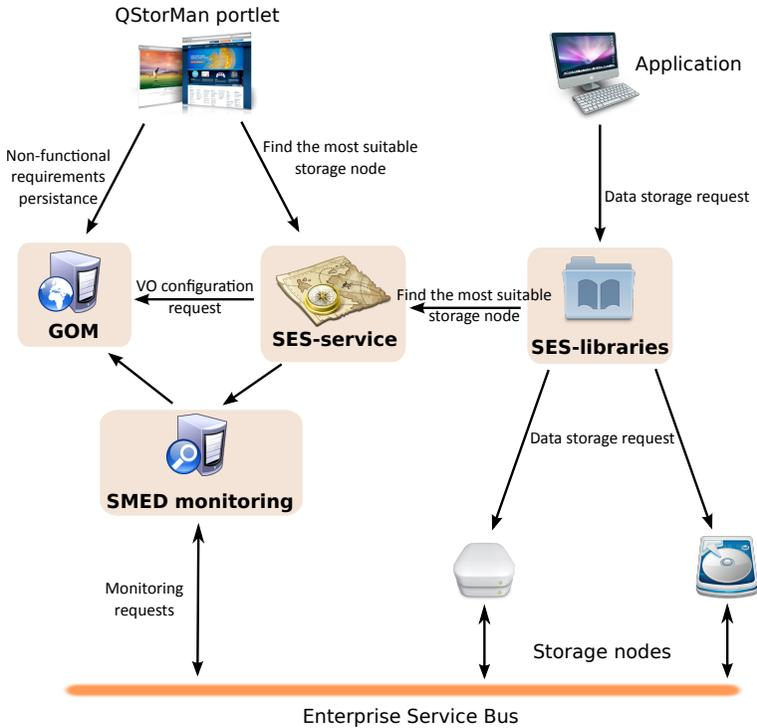
Fig. 1. The architecture of the QStorMan toolkit
