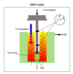
Fig. 1. Melt volume rate determination [22]
