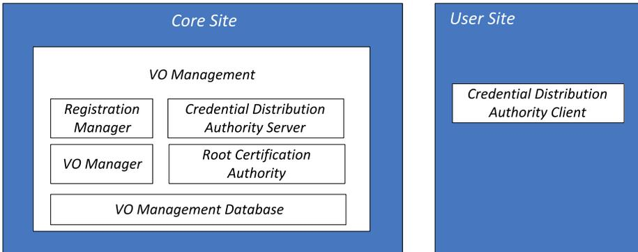
Figure 4. Structure of the XtreamOS VO management service
