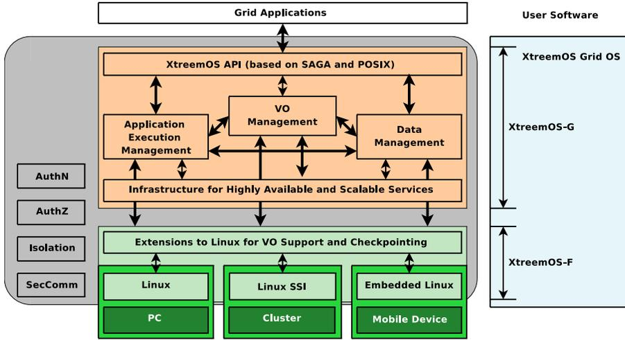
Figure 1. XtremOS software architecture [6]
