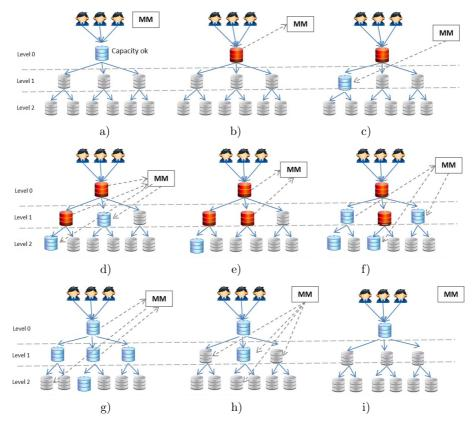
Figure 3. Resources use for the proposed system: a) Initial state, b) Maximum capacity, Send notification, c) Activate node from the next level, d) Still maximum capacity, activate another node in the next level, e) Maximum capacity, Send notification, f) Minimum capacity, Send notification, g) Minimum capacity, Send notification, Shutdown server in lowest level, h) Shutdown the unnecessary servers, i) Shutdown the unnecessary servers
