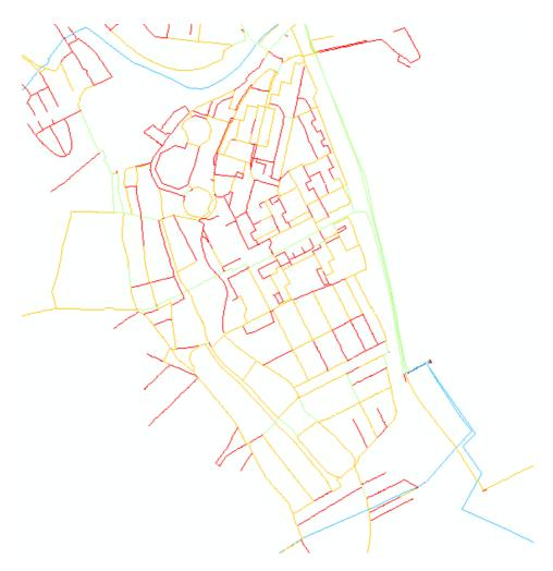
Figure 9. Water velocity (m/s) on pipe links by color range indicators
