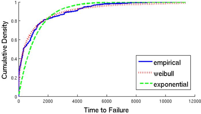
Figure 4. Time-to-failure distribution of a machine after filtering out periodic failures and its fitting to Weibull and exponential distributions
