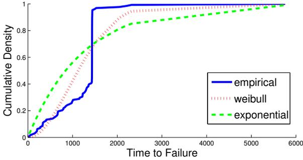
Figure 2. The distribution of a machine’s time-to-failure modeled using the Weibull and the exponential distribution
