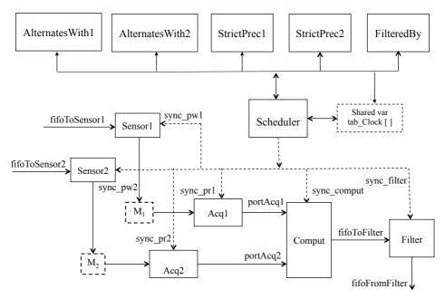
Figure 9. Structure of the generated FIACRE code
