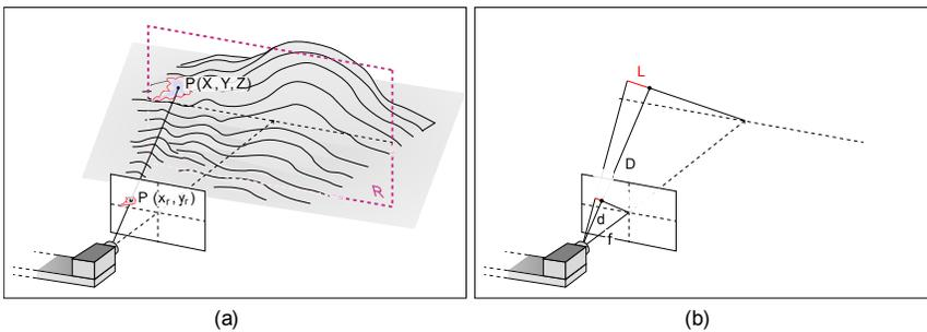
Figure 4. Calculating pixel coverage using: a) the relation between the point  $P(X, Y, Z)$  in the real world and  $P'(x_r, y_r)$  in the image plane, and b) the relation between shift  $L$  in the real world and the shift  $l$  in the image plane
