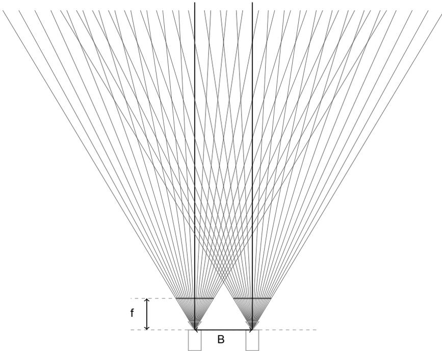
Figure 2. The discretization error as the result of the discrete nature of the imaging system. Diamond shapes represent uncertainty areas, i.e., the system returns the same distance for all the points inside the same diamond region.
