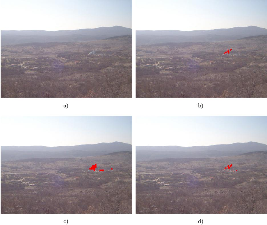
Figure 8. a) Input image with visible smoke, taken by the right stereo camera, b) image with smoke detected by *Method 1*, c) image with smoke detected by *Method 2*, d) image with smoke detected by *Method 3*
