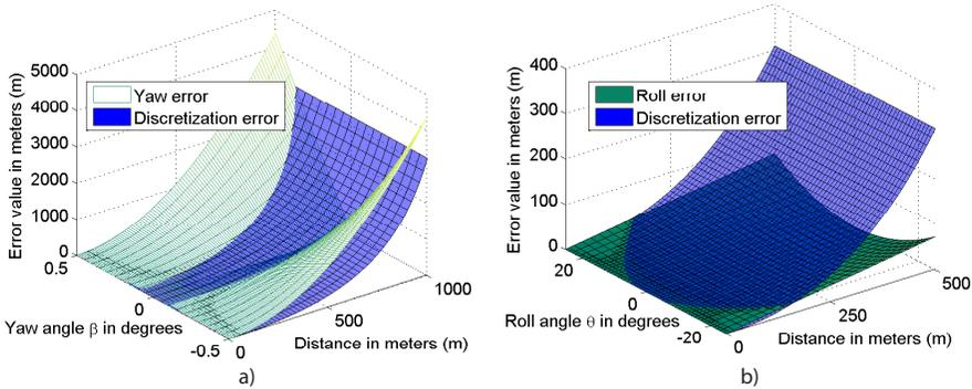
Figure 3. a) Absolute yaw error  $|Z_{yaw\_err}|$  (green), and maximum absolute discretization error  $Z_{disc\_err}$  (purple), b) absolute roll error  $|Z_{roll\_err}|$  (green), and maximum absolute discretization error  $Z_{disc\_err}$  (purple) (for a stereo system with  $B = 2$  m,  $f = 4.655$  mm,  $x_{pix} = 0.0071$  mm, and  $X2 = 3$  m)
