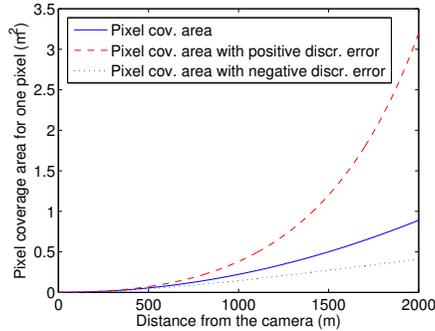
Figure 5. Pixel coverage area ( $\text{m}^2$ ) for one pixel with regard to the distance from the camera (blue solid line), pixel coverage area with maximum positive discretization error for the given distance (red dashed line), and pixel coverage area with maximum negative discretization error for the given distance (black dotted line). The selected pixel has coordinates (100, 100) referent to the center of the image, with  $B = 2$  m,  $f = 4.655$  mm and  $x_{pix} = 0.0022$  mm.
