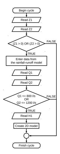
Figure 7. Algoritm for assessment of the flood possibility
