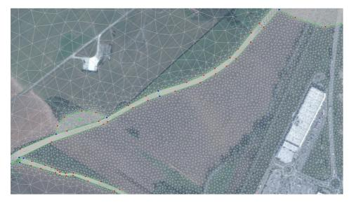
Figure 4. Partial computation mesh of the created two-dimensional mathematical model
