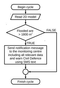
Figure 9. Notification decision algorithm of the local flood warning system
