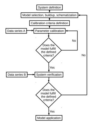
Figure 6. Schematic representation of the steps taken during the calibration and verification of the model
